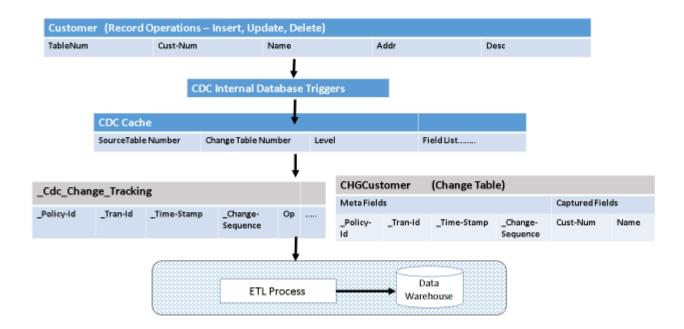
The data captured by the CDC triggers reflects the source records after they have been modified. The action of capturing the data is stored in the system wide Change Tracking Table. The captured data is then stored in a source specific Change Table.
